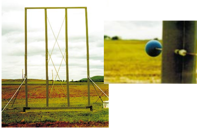
Fig. 1. Left: Fiberglass beams and anchors used to support the microphone array. Right: Close-up view of a microphone and the mounting bracket. Readers of the print version should refer to the color version of these pictures in the online archival version.
